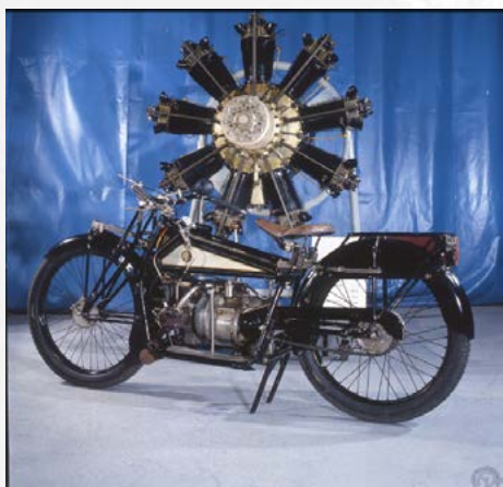
1922 Gnome & Rhône ABC/Type A. Nine-cylinder 60 HP rotary engine – the last operational radial engine of this type built in 1920 Photo credits: moto-collection.org Dominque Fradin
